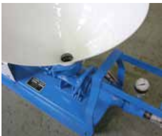
Funnel hopper and pressure gauge
